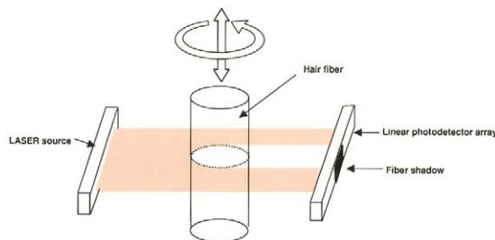
Fig 4. Device used for geometry and morphology analysis.
