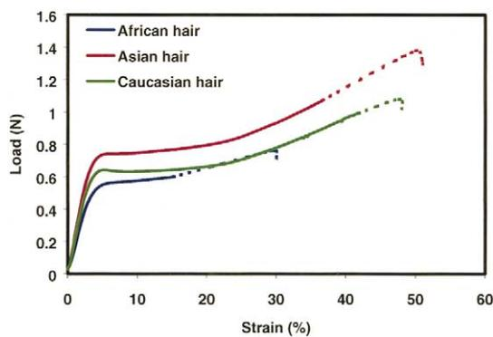
**Fig 5.** Load and strain curves of African, Asian, and Caucasian hair.
